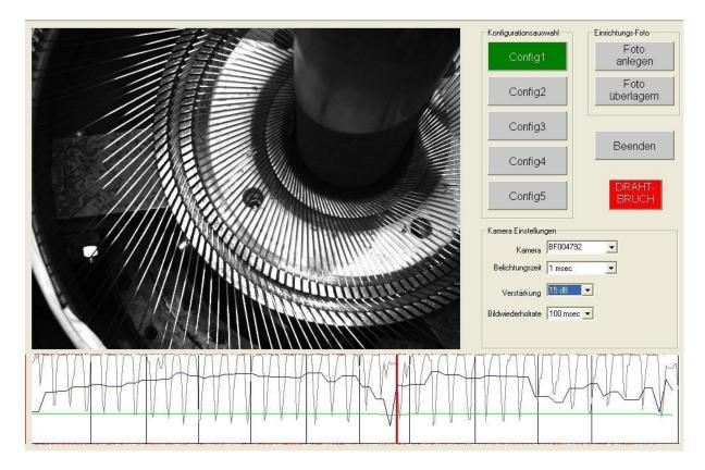
The rotating reel disc is viewed by a camera. At times, the camera is covered by a revolving satelite system which is providing an insulating layer for the next step.
